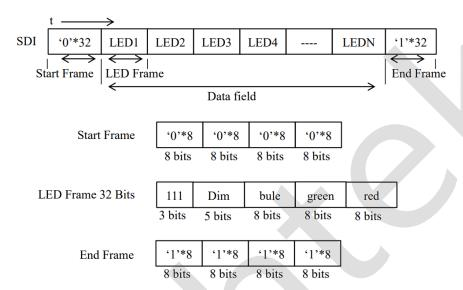
1.1 5-Bit Brightness Adjustment and Specification Limits
