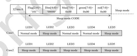
In Case 1, if LED 2 is in sleep mode, during the subsequent data transfer process, the state of LED 2 will remain unchanged as long as 32 bits of data for LED 2 is received with Flag[2:0], DIMMING[4:0] set as 8h"A0". This indicates that LED 2 will remain in sleep mode. In this scenario, LED 2 can relay the remaining 32 bits of data to LED 3 to modify the display data of LED 3. In essence, the inactive chip (LED 2 in sleep mode) has the capability to relay data to the subsequent chips.
