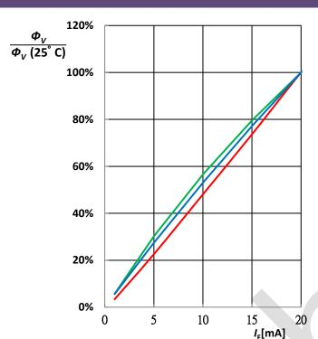
Relative Intensity vs. Temperature  $\Phi_V/\Phi_V$  (25°C) = f(I<sub>F</sub>); T<sub>S</sub> = 25 °C;
